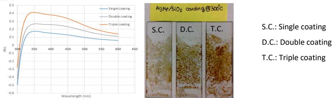
Fig. 1 Different layers of Silver nanoparticle/silica coating
