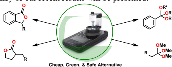
Fig. 1 Electrosynthesis of pharmaceutically desirable small molecules using the IKA Electrasyn
